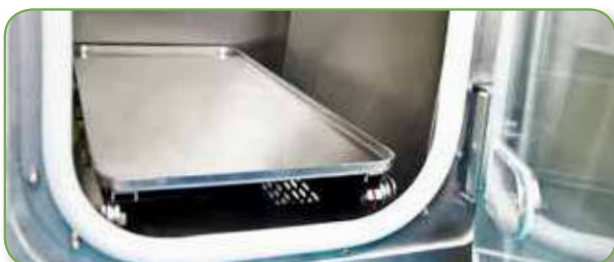
Horizontal sliding tray prevents operator fatigue during transfer procedures
